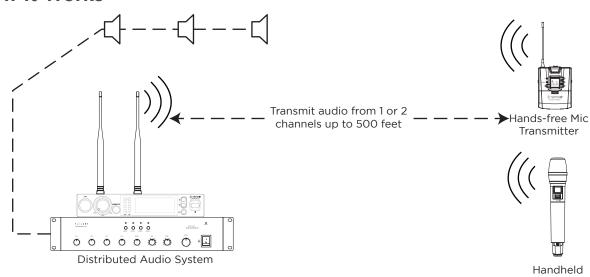
The wireless receiver can be placed on a surface or mounted in a rack. The antennas can be mounted in the front, rear, or extended with an antenna booster (sold separately) for wireless sound pick up from a hand-held microphone transmitter or a hands-free body pack (see below for full list of accessories). The SE-350-WR-1CHD receives transmissions up to 500 feet, then outputs into a distributed audio system.
