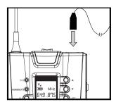
Connect the 4 pin mini-XLR cable into the "MIC IN" of the body pack.
